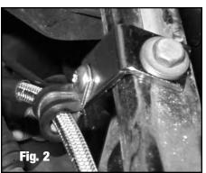
Fasten hose and ABS wire to top of knuckle using factory bolt and supplied cushion clamps. NOTE: For best results, tap front hole on right (passenger) side knuckle for M6 x 1.0 thread to locate hose and ABS wire (See Figure 3).
