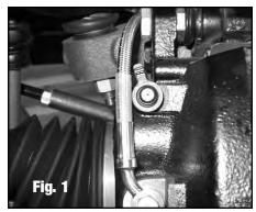
Install short end of "L" bracket onto top of upper A-arm using factory bolt. Install cushion clamp onto hose and attach to long end of "L" bracket using supplied nut and bolt (See Figure 2).
