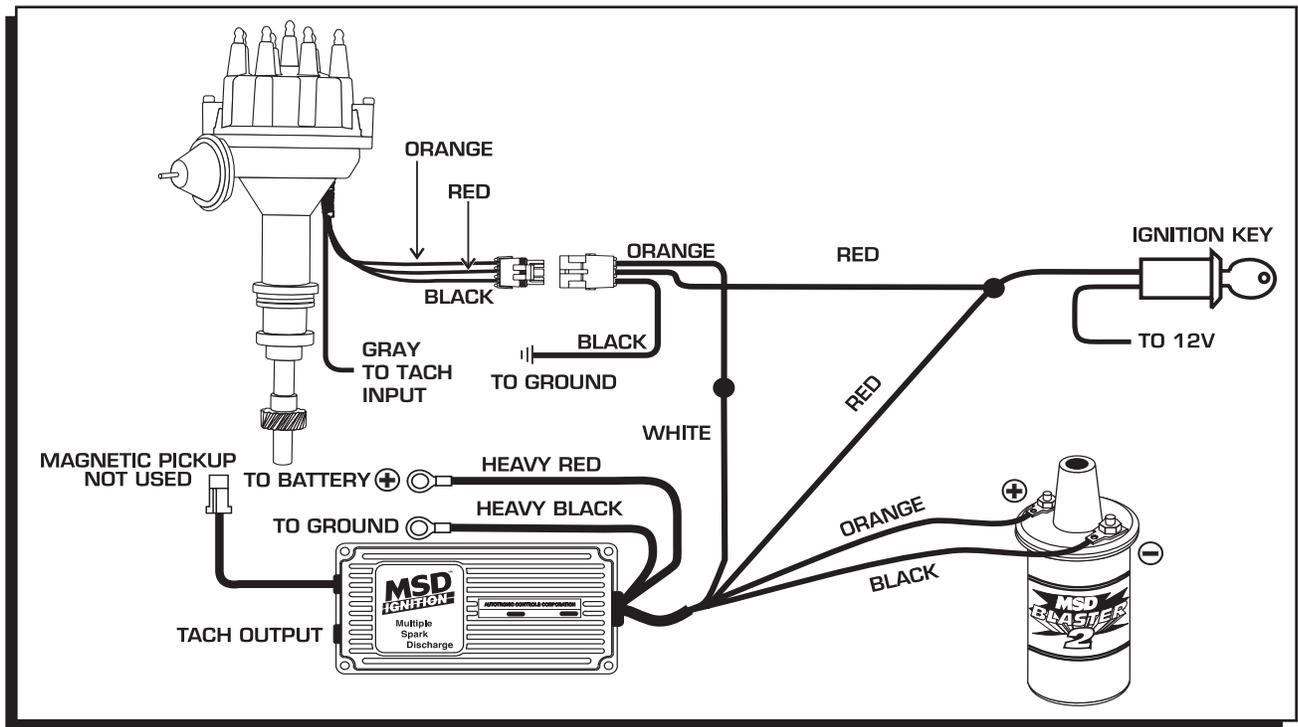
Figure 13 Wiring to an MSD Ignition Control.
