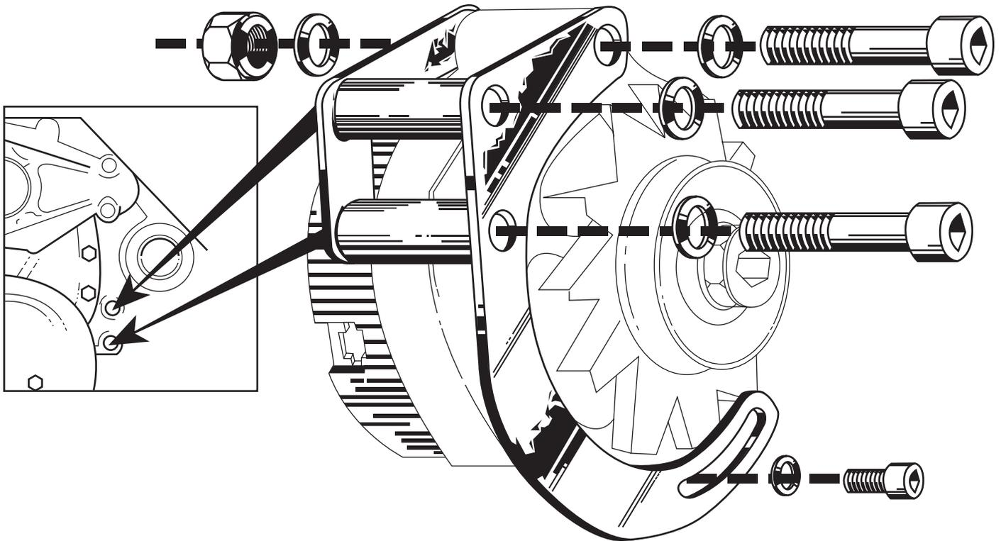
**NOTE:** Alternator wiring location and length may need to be altered depending on current alternator position.
