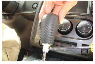
Friction Snap – With a small flat-tip screwdriver, carefully spread the locking fingers apart while pulling the shifter handle upward, until the handle comes free.
