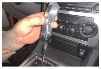
6. Slip the handle body onto the shifter stick.
