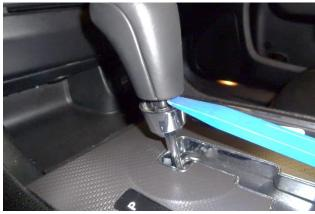
If your shifter handle is not threaded, carefully pry the chrome trim ring off the shifter handle. This will reveal the how your handle is attached. NOTE: Do not pry the trim ring off threaded shifter handles!
