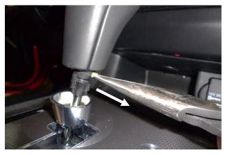
4. **Spring Clip** – Use pliers to pull the spring clip out of the shifter handle, then lift the handle off the shifter stick.
