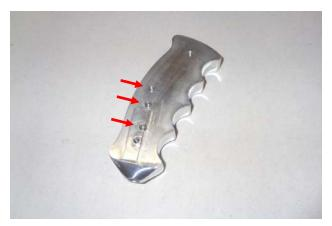
5. Install 3 set screws (Item 6) on each side of the shifter handle body (1). Leave about 1 or 2 threads showing.
