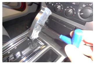
7. Properly align the shift handle, then tighten all six set screws.
