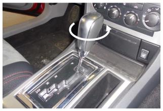
Threaded – Threaded shifter handles simply twist off the shifter stick in a counterclockwise direction.
