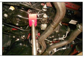
4. Remove the lower bolt from the rear shock.
