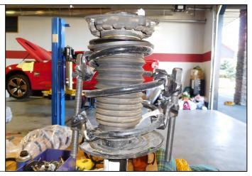
25. Once the upper cup no longer has tension from the spring, remove the nut holding the upper cup in position. A strap wrench may be needed to hold the shaft of the shock to allow the locking nut to be removed.
