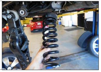
10. Remove the factory spring rubber from the top and bottom of the spring.
