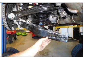
9. Once the spring moves freely, remove the jack and let the rear control arm swing out of the way, while holding onto the spring.
