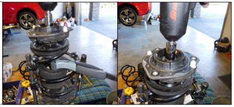
26. Remove the upper cup and rubber boot before removing the spring.
