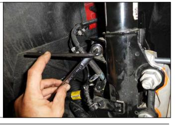
18. Remove the spindle assembly nuts from the bolts only. Do not turn the bolts.
