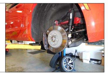
2. Remove the four plastic rear clips that mount the plastic control arm covers by pushing down on the center pin, then remove the covers.
