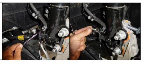
17. Remove the upper sway bar link using a box end wrench with an allen wrench. Once the nut is removed, slide the threaded end of the sway bar link out of the strut assembly.
