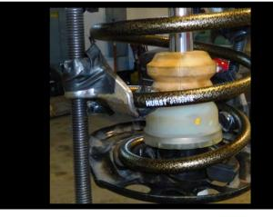
30. Also note that the upper cup assembly has no special alignment for the top of the spring. The upper cup assembly can be installed without any alignment marks.
