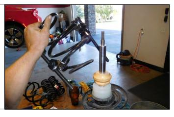
28. Install your new Hurst spring in the reverse order of removal. Take note of the rubber isolator on the strut assy. Align the new spring making sure it seats properly.
