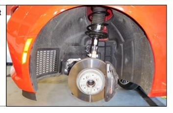
15. Install a M10/1.50 bolt into the upper portion of the spindle assembly until it makes contact with the strut. Use a nut to lock the bolt into position. This sets the alignment angles for re-assembly. Vehicle alignment is still needed.
