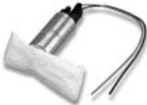
Our electric in-tank line offers coverage for the most popular Ford, Chrysler, GM and Import applications. Utilizing a proven gerotor design, these pumps are available in either a 190 or 255 liter per hour (lph) flow rate.
