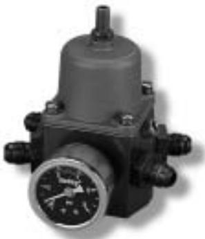
**INSTALLATION TIP** - for vehicles without fuel return line to the tank: Install the regulator close to the carburetor. Fuel lines from the regulator to the carburetor should be #6 (3/8").
