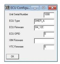
To take advantage of the newest features, use the new C-Com® software and make sure the ECU has 12C (or later) firmware loaded. When using an existing tune, several forms and tables need to be accessed through the new C-Com® software to make sure they have appropriate values entered.
