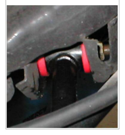
17507 06/MAR/07 BPL GREASE ALL PARTS THAT COME INTO CONTACT WITH POLYURETHANE
