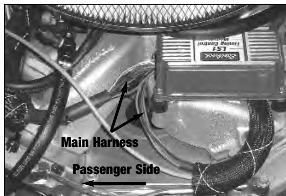
Figure 4 - Timing Control Module Mounting
