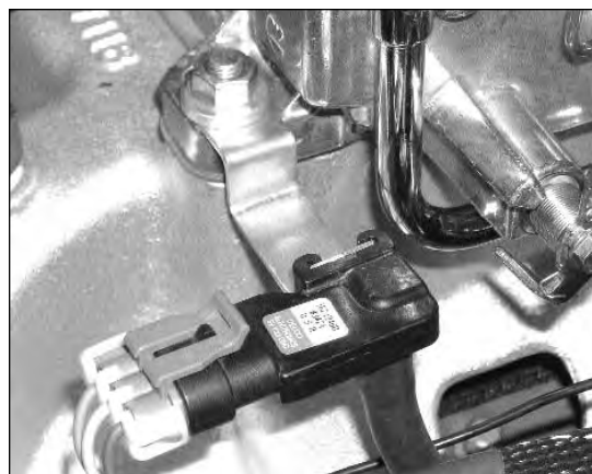
Figure 3 - Map Sensor and Bracket
