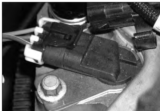
Figure 6 - Camshaft Position Sensor
