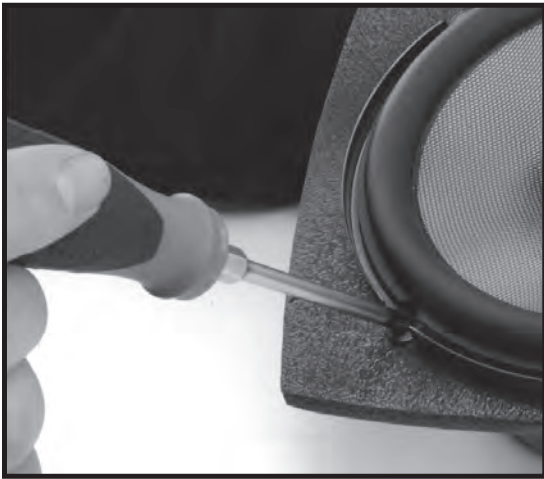
Fig 4 - Make small holes for mounting screws
