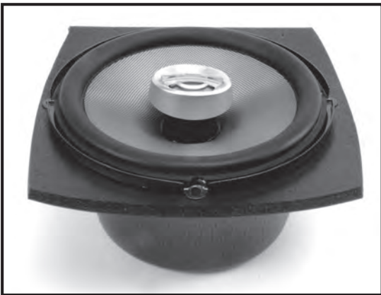
Fig 1 - Test fit speaker into baffle
