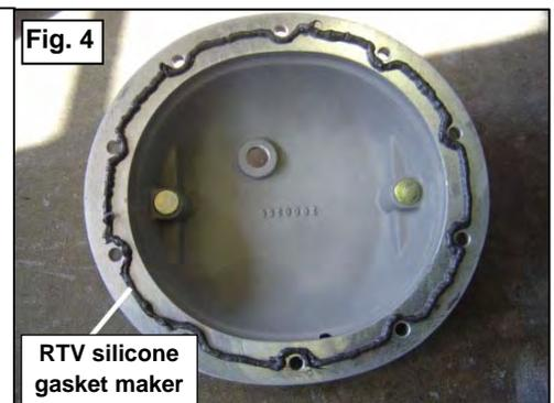
12. Install the B&M Cast Aluminum Differential Cover on the axle housing using a supplied bolt and washer at a bottom hole on the cover so it can be used as a guide.
