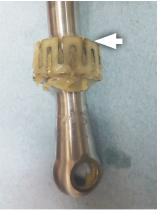
14. After thoroughly cleaning ball seat, lubricate with grease (5) and fit it onto short throw shifter (1) (notches facing up) as shown.
