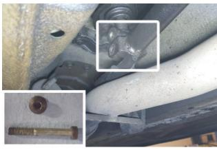
Remove nut and bolt attaching shift lever to change rod. Carefully lower change rod and allow it to hang out of the way.
