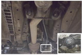
**NOTE:** Shifter must be carefully guided into mount to keep it from ripping dust seal – take your time.
