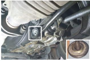
7. Remove bolt holding front of change extension to transmission.
