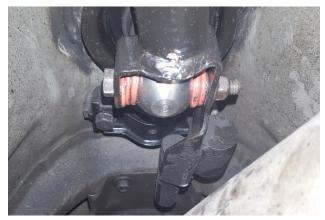
23. Insert bolt and tighten nut to 16 ft-lbs.
