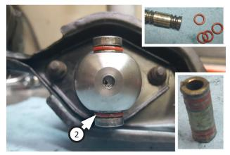
18. Thoroughly clean rear joint collar and assemble (x4) **o-rings (2)** into grooves. Again, lubricate joint collar, bushings and hole in bottom end of shifter. Install joint collar into hole in shifter.
