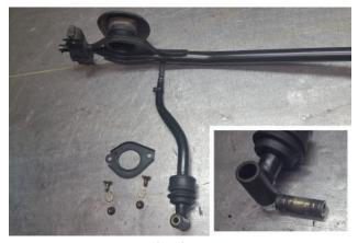
11. Index orientation of shift lever then separate it from change extension. Then remove rear joint collar as shown.
