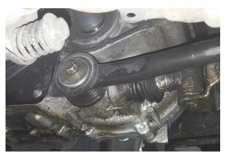
20. Remount front of change extension to transmission and tighten bolt (removed step 7) to 16 ft-lbs.
