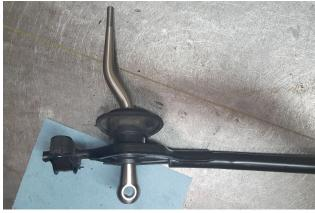
**NOTE:** If installing a curved stick, orient it exactly as the original shifter was.
