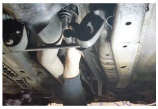
8. Carefully pull change extension and shift lever from vehicle.
