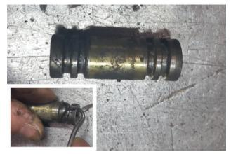
12. Remove (x4) o-rings from rear joint collar then wipe away any excess grease.
