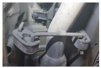
4. If you can't easily access your change rod, unhook rubber exhaust hangers near catalytic converter and carefully lower exhaust pipe.
