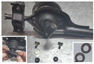
10. Remove (x2) change ball fasteners and holder from shift lever. Retain them for later use. Pull rubber rings from joint collar.
