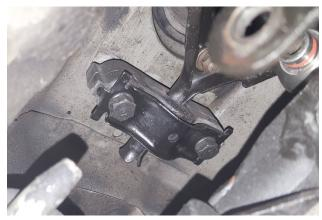
21. Remount rear of change extension into rear extension mount, then replace (x2) bolts (removed step 6) and tighten to 16 ft-lbs.
