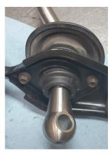
17. Replace change ball holder carefully working dust seal lip back into opening. Fasten holder with fasteners, (removed step 10) making sure square potion of bolt is fully seated. Tighten to 7 ft-lbs.
