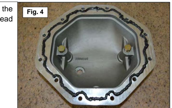
12. Install the B&M Cast Aluminum Rear End Cover on the axle housing using a supplied bolt and washer at a bottom hole on the cover so it can be used as a guide.
